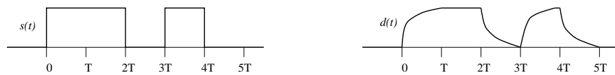
Figure 4. The relation between input and output waveforms for transmission channel with filtering
