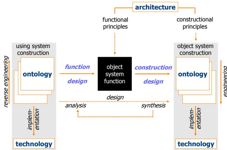
Figure 1 Generic System Development Process (after Dietz 2005 p. 23)
